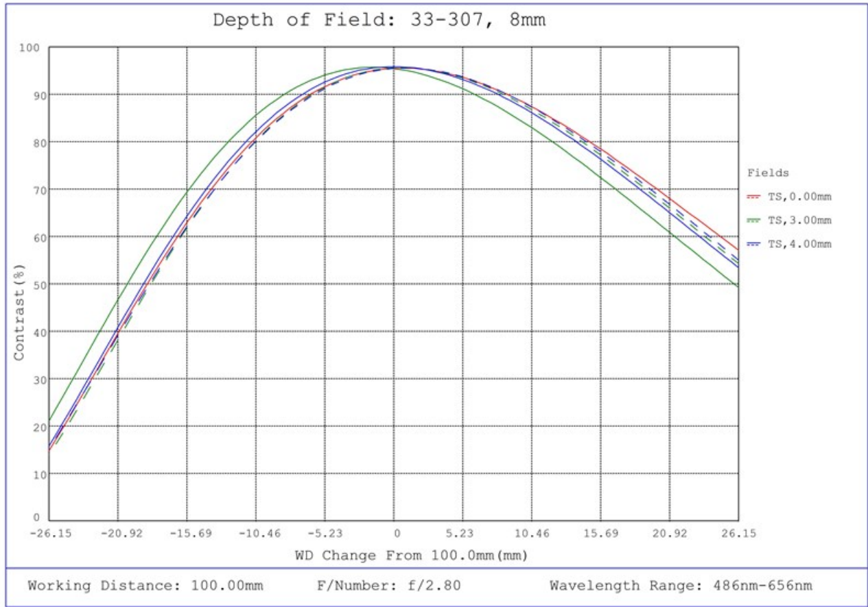
#33-307, 8mm UC Series Fixed Focal Length Lens, Depth of Field Plot, 100mm Working Distance, f2.8
