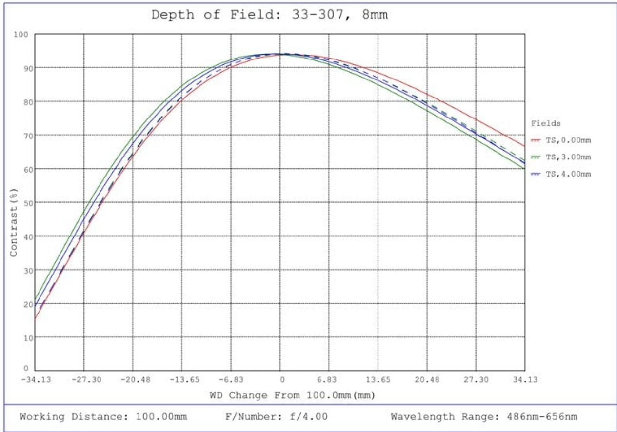
#33-307, 8mm UC Series Fixed Focal Length Lens, Depth of Field Plot, 100mm Working Distance, f4
