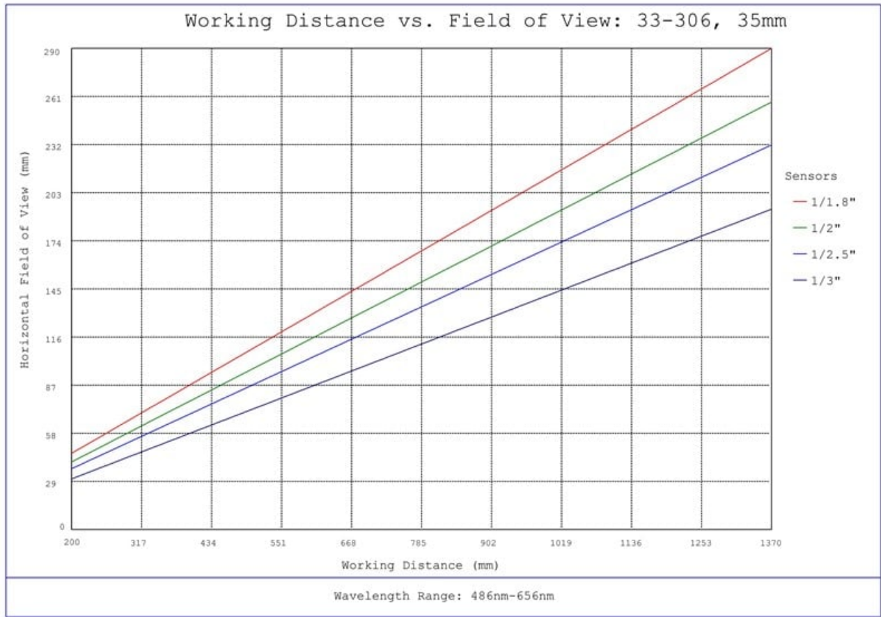
#33-306, 35mm UC Series Fixed Focal Length Lens, Working Distance versus Field of View Plot
