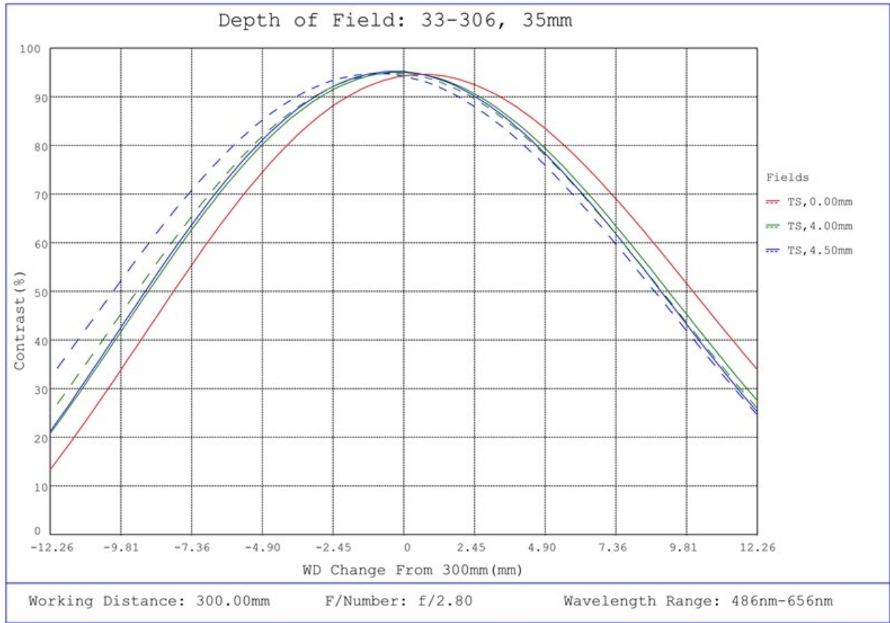
#33-306, 35mm UC Series Fixed Focal Length Lens, Depth of Field Plot, 300mm Working Distance, f2.8
