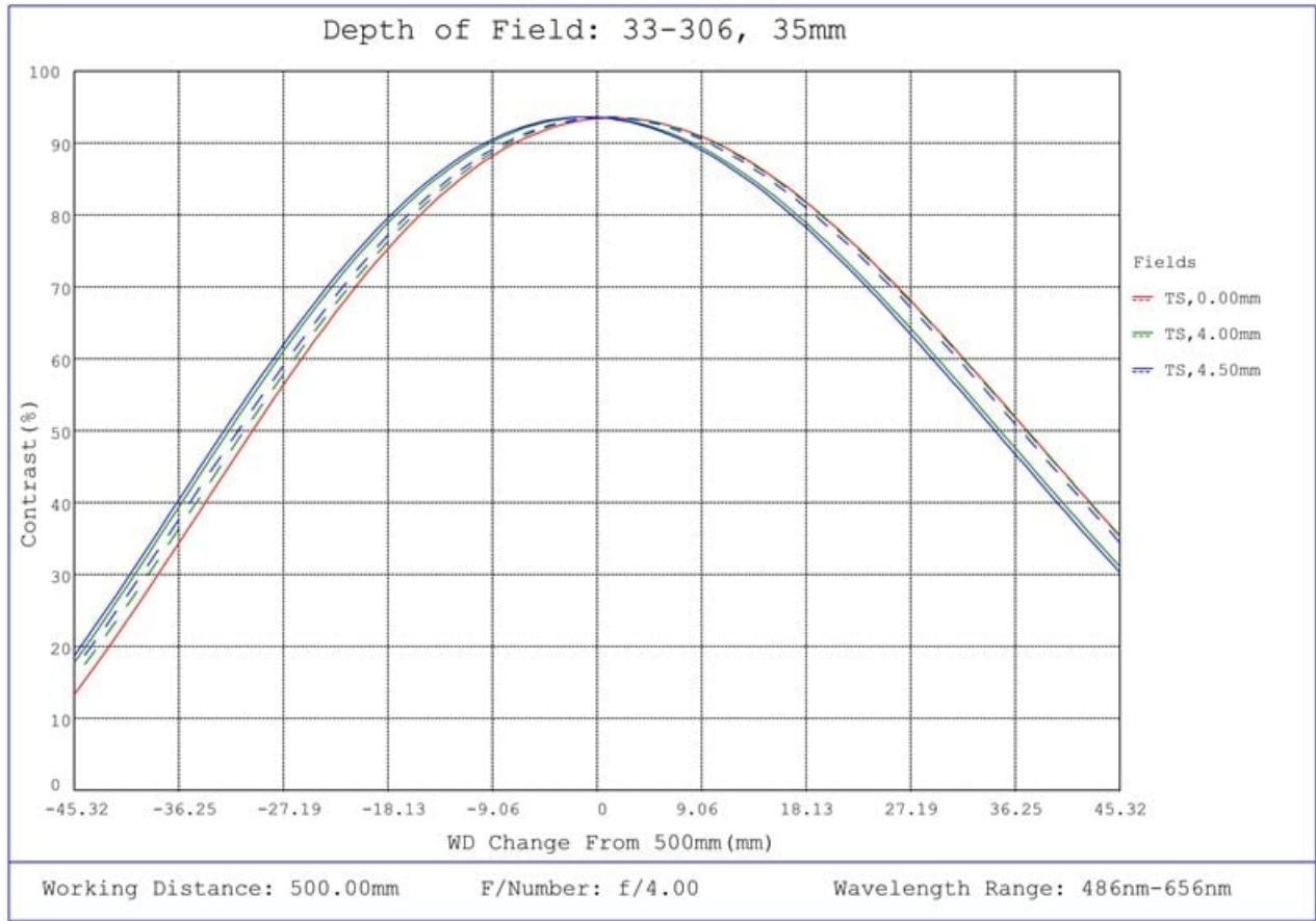
#33-306, 35mm UC Series Fixed Focal Length Lens, Depth of Field Plot, 500mm Working Distance, f4
