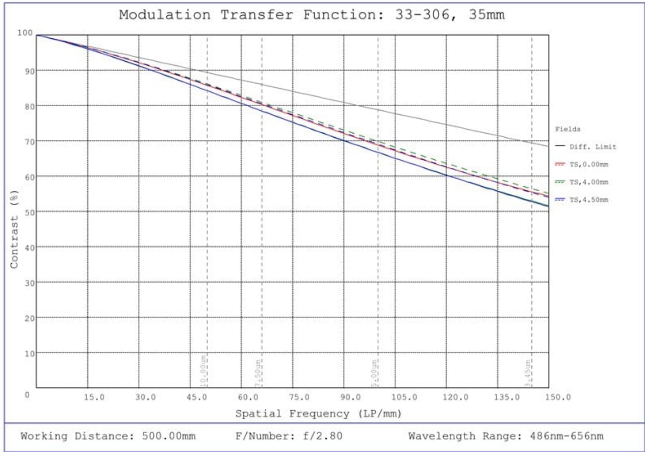
#33-306, 35mm UC Series Fixed Focal Length Lens, Modulated Transfer Function (MTF) Plot, 500mm Working Distance, f2.8
