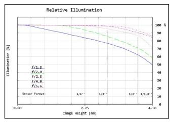
Figure 2: Relative illumination (center to corner)
