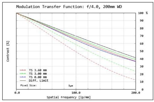
Figure 7: Image space polychromatic diffraction FFT Modulation Transfer Function (MTF) for  $\lambda = 486$ nm to 656nm. Included are Tangential and Sagittal values for field points on center, at 70% of full field and at the maximum sensor format. Solid black line indicates diffraction limit determined by f/#-defined aperture. Frequencies corresponding to the Nyquist resolution limit of pixel sizes are indicated.
