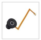
This **C-module** integrates a fixed lens module and an A-39N0 Variable Focus Lens in an M12 receptacle (S-mount). The module is built-in with an FPC cable, and can be connected to a standard 1 mm pitch FPC connector. It can therefore be very easily integrated in a standard M12 sensor board. The module is compatible with imaging sensor formats up to 1/3" diagonal. This module can be driven by the same drivers as the A-39N0 lens.
