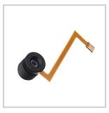
This **C-module** integrates a fixed lens module and an A-25H0 Variable Focus Lens in an M12 receptacle (S-mount). The module is built-in with an FPC cable, and can be connected to a standard 1 mm pitch FPC connector. It can therefore be very easily integrated in a standard M12 sensor board. The module is compatible with most imaging sensor formats, from 1/4" to 1/1.8" diagonal. This module can be driven by the same drivers as the A-25H0 lens.
