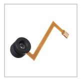
This **C-module** integrates a fixed lens module and an A-25H0 Variable Focus Lens in an M12 receptacle (S-mount). The module is built-in with an FPC cable, and can be connected to a standard 1 mm pitch FPC connector. It can therefore be very easily integrated in a standard M12 sensor board. The module is compatible with most imaging sensor formats, from 1/4" to 1/2.5" diagonal. This module can be driven by the same drivers as the A-25H0 lens.
