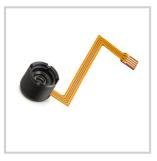
This **C-module** integrates a fixed lens module and an A-25H0 Variable Focus Lens in an M12 receptacle (S-mount). The module is built-in with an FPC cable, and can be connected to a standard 1 mm pitch FPC connector. It can therefore be very easily integrated in a standard M12 sensor board. The module is compatible with most imaging sensor formats, up to 1/2.4" diagonal. This module can be driven by the same drivers as the A-25H0 lens.
