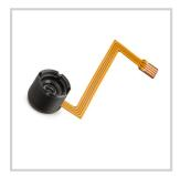
This **C-module** integrates a fixed lens module and an A-25H0 Variable Focus Lens in an M12 receptacle (S-mount). The module is built-in with an FPC cable, and can be connected to a standard 1 mm pitch FPC connector. It can therefore be very easily integrated in a standard M12 sensor board. The module is compatible with most imaging sensor formats, up to 1/3" diagonal. This module can be driven by the same drivers as the A-25H0 lens.
