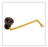
This **C-module** integrates a fixed lens module and an A-25H0 Variable Focus Lens in an M12 receptacle (S-mount). The module is built-in with an FPC cable, and can be connected to a standard 1 mm pitch FPC connector. It can therefore be very easily integrated in a standard M12 sensor board. The module is compatible with imaging sensor formats up to 1/2.5" diagonal. This module can be driven by the same drivers as the A-25H0 lens.
